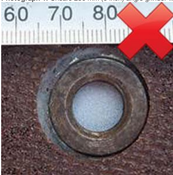
Photograph 2: Unsafe excessive clearance for the central hole on 356 mm disc on 9 inch spindle flange.
