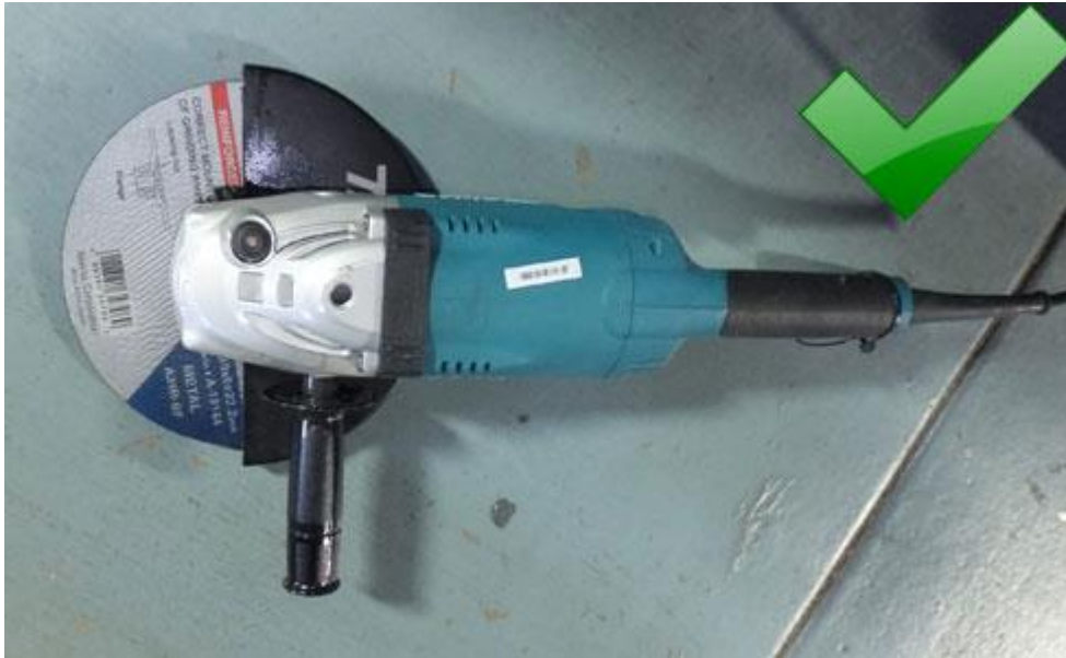
Photograph 3: 230 mm (9 inch) angle grinder with guard and right sized disc fitted.
