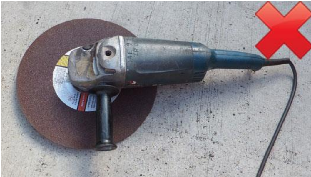
Photograph 1: Unsafe 230 mm (9 inch) angle grinder with 356 mm (14 inch) disc fitted and guard removed.
