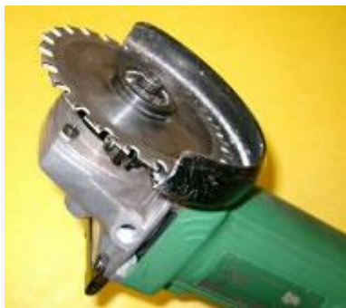
Photograph 1 - multi-cutter fitted to a 100mm angle grinder
