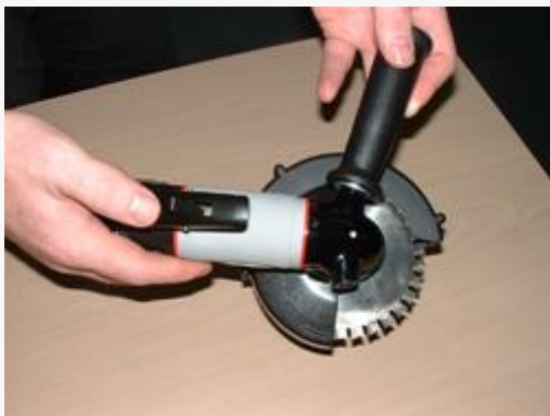
Photograph 2 - multi-cutter fitted with full spring loaded guarding (closed)
