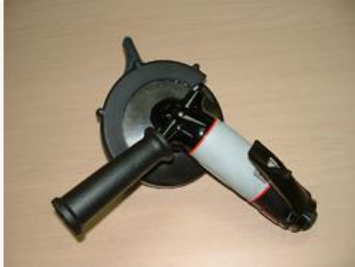
Photograph 2 - multi-cutter fitted with full spring loaded guarding (closed)
